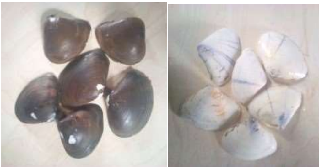
Fig. 1: Waste clam shells before Washing/drying Fig. 2: Waste clam shells after washing/drying
