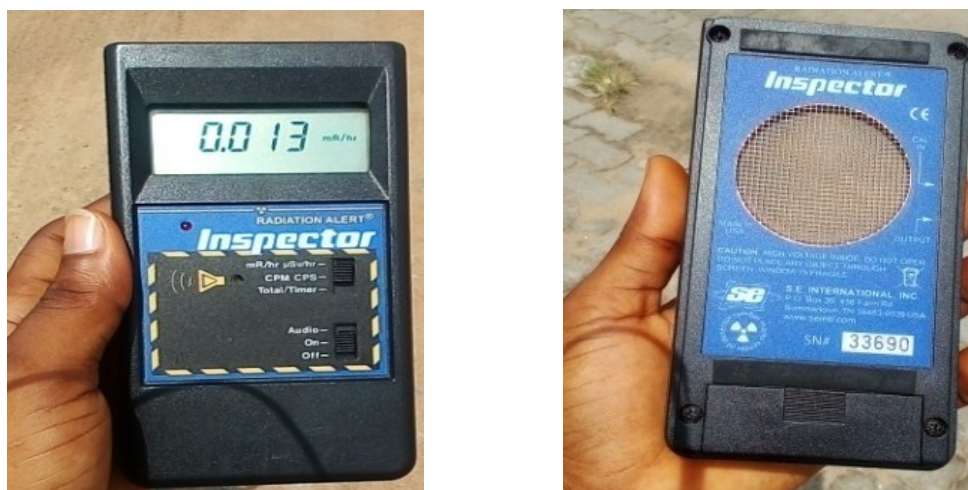
Fig 1: Back and Front view of the Radiation Monitoring Device- Radalert x100.
